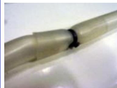
Crimp and push the end of the new bladder tube 30-40 mm inside the old tube, and secure with a tight ligature of rubber or cord (do not use metal wire).
