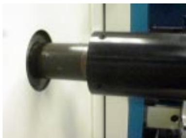
Release the drive end cover lock screws and slip the cover back, away from the slip rings, to expose the bladder clamps in the four slots. Remove the outer end cover as shown in the previous section.
