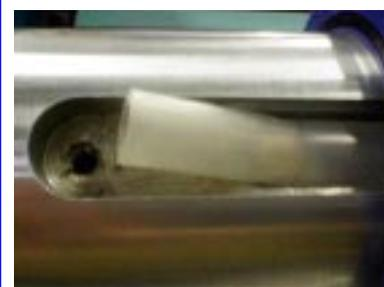
Trim the new tube as shown above and mark the air hole position with a ball point pen. Using a 3mm dia drill between the fingers, carefully make a hole in one side of the tube. Insert the Air Clamp screw and washer and gently tighten - do not overclamp!
