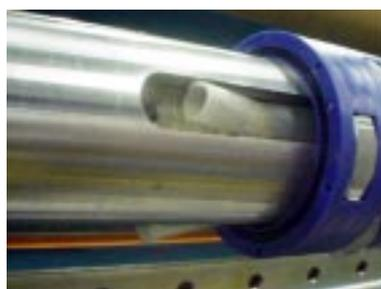
Slide two Slip ring units over the free end of the bladder to expose the Air entry clamp screw. (Note Pressure shoes will be released as the Skip rings are moved). Remove the Air entry clamp screws (as shown opposite).
