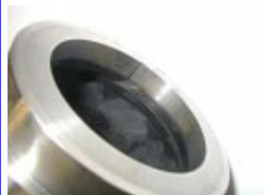
**Note! the spring seal opening on 6" chucks should be arranged about the keyway**
