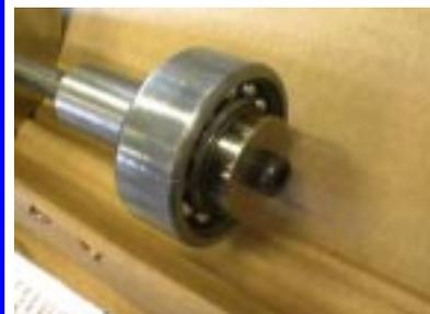
Bearing fitted on stub shaft
