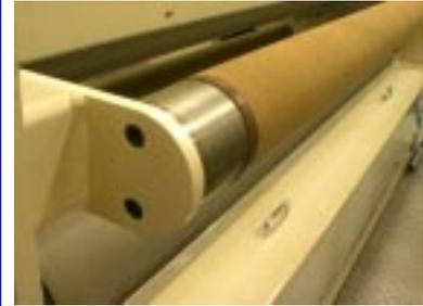
Typical Idle roller in place, showing the two retaining screws
