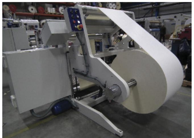
Heavy duty unwind stands to allow large reels of material to be run for further continuous running capabilities with servo web guide systems and reel lifts built in.
