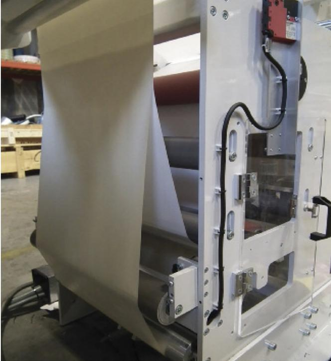
Delam/Relam system to allow difficult adhesive materials to matrix strip with ease at speed. Adjustable for various substrates.
