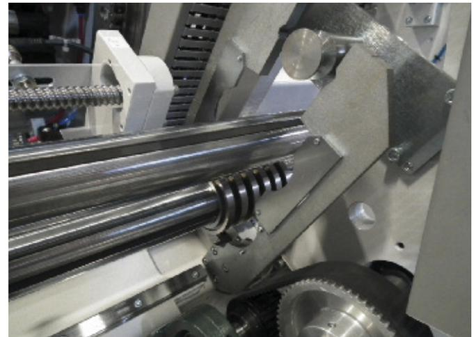
Automatic knife positioning system upgrade to allow up to 20 knife sets to be set by 3 x operator parameter settings. 6 x knives set in 90 seconds typically.
