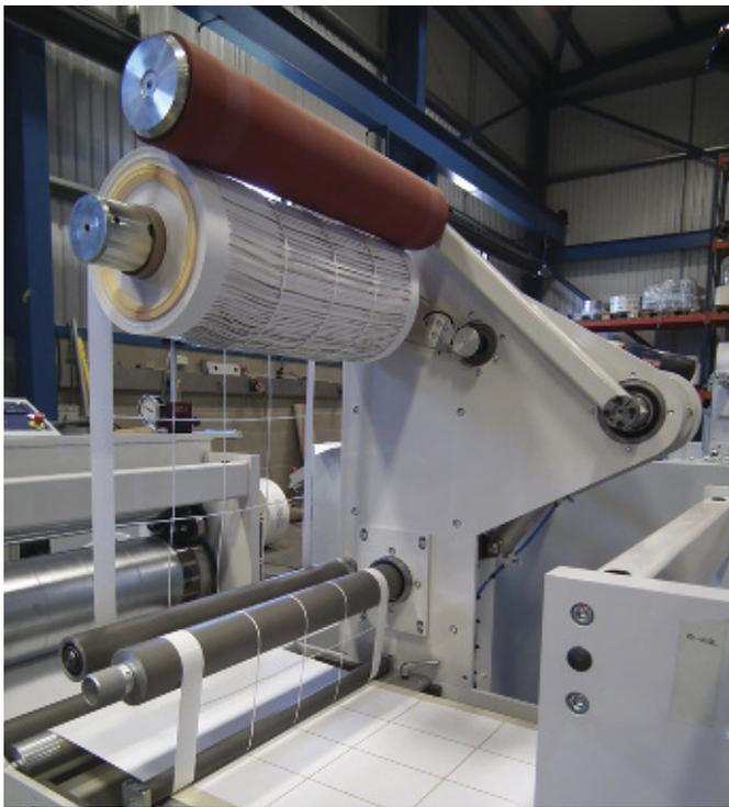
Matrix waste winder pneumatically loaded lay on roller assembly for special shaped labels to allow continuous operation.
