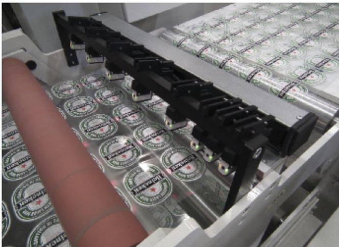
Various types of missing label detection systems available for different substrates. Easy positioning system to suit varying label width.
