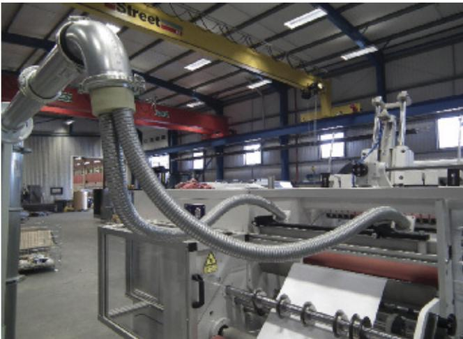
Edge trim extraction systems available to be designed with the complete machine. Simple air jets or high speed VENTURI systems used.
