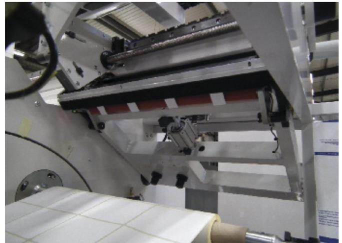
Tail closure via label with option to print facility to give reels completely glue free concept.
