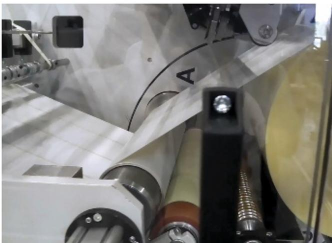
Patented GLUE-LESS design for reels of labels glue free with no attachment to the paper or plastic core.
