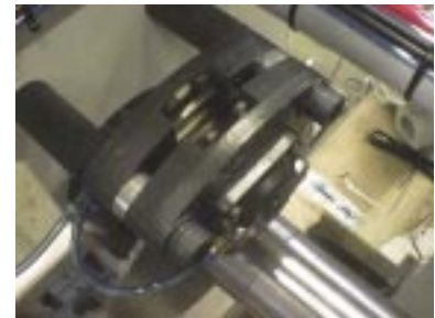
Almatic Disk Brake Both pads in place
