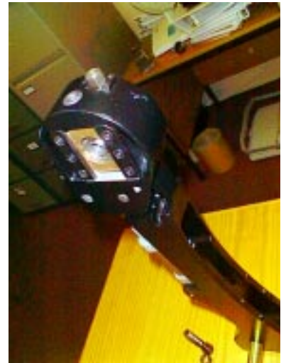
The adjustable spherical bearing carriage is retained by six countersunk socket screws.
