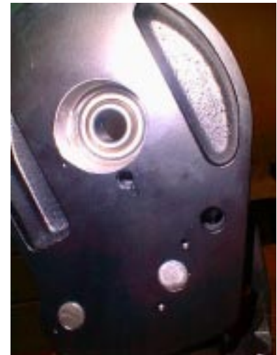
The fixed spherical bearing is retained by a circlip
