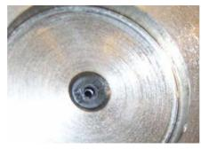
Remove the retaining socket grub screws, and withdraw end plug using a slide hammer on a suitable stud.
